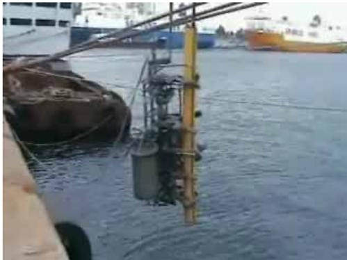
Flexible riser Inspection System – Robot crawler
